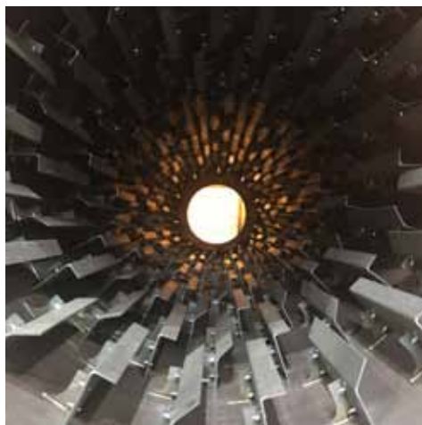
HP Rotary Dryer Internal Flighting
